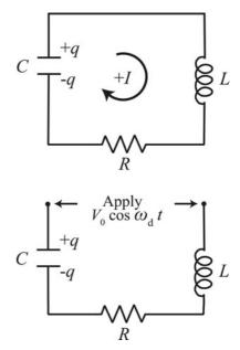
Figure 4.6.1 Top: RLC Oscillator. Bottom: Driven RLC oscillator.
