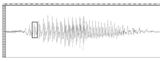
**Figure 9.12.3** The word "Hi!" as recorded with a microphone. The vertical axis is proportional to the variation in air pressure relative to background, while the horizontal axis is time in s.
