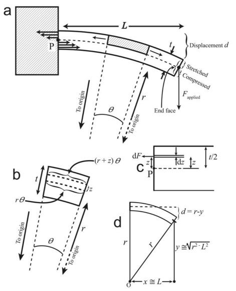
**Figure 2.6.1** a: A cantilever is bent. The top half is stretched, while the bottom half is compressed. The highlighted segment must feel equal forces from the left and right. b: Enlarged view of a section of the cantilever. c: Enlarged view of the end of the cantilever that is attached to the wall. d: Relation between displacement and radius of curvature.
