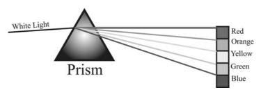
Figure 10.P.4 A prism is used to separate white light into beams of different wavelengths.
