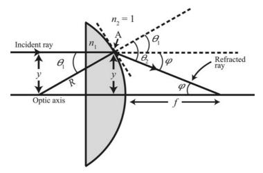
Figure 10.8.2 Refraction for a plano-convex lens.
