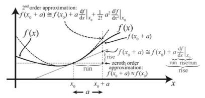
**Figure 1.6.1** Graphical illustration of the Taylor series approximation.
