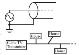
Figure 10.3.1 Top: model for a cable TV transmitter attached to a coaxial cable.
