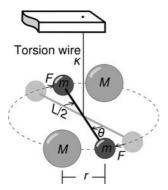
**Figure 2.5.2** Schematic diagram of the Cavendish experiment. (Figure by Chris Burks.)
