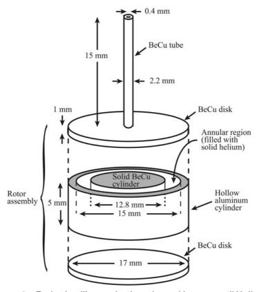
Figure 2.P.2 Torsional oscillator used to detect the transition to supersolid helium.
