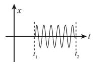
Figure 1.12.1 Motion of one point on a piano string.
