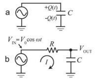
**Figure 1.10.2** a: A signal generator connected to a capacitor. b: An RC low-pass filter.
