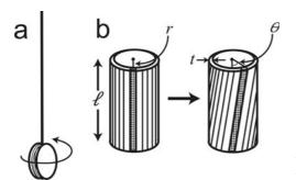
**Figure 2.5.1** a: A yo-yo twisting on the end of its string. b: Twisting a thin-walled tube.
