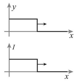
Figure 10.5.3 When you first apply a voltage to the left end of a transmission line, you generating a wavefront in the voltage which propagates down the line, accompanied by a wavefront in the current.
