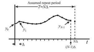
Figure 8.6.1 Sampling a continuous waveform, in preparation for the DFT.
