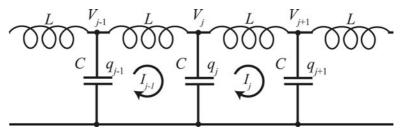
Figure 9.7.1 Model for a transmission line.
